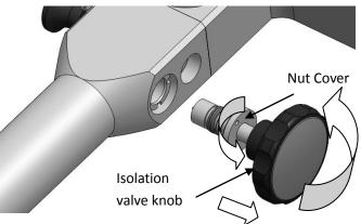
Turn the isolation valve counterclockwise to about half way out.
