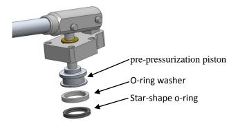
A. Remove the start-shape o-ring (21.82X3.53) from pre-pressurization piston. Replace the o-ring, and assemble all parts back in reverse order.
